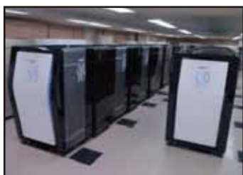
Supercomputer system NEC SX-9 × 10 nodes Total processing capacity: 16TFLOPS Total memory: 10TB
