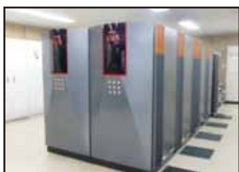
Supercomputer system NEC SX-8R × 20 nodes Total processing capacity: 5.3TFLOPS Total memory: 3.3TB
